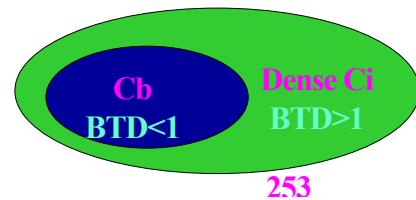
Figure 1. Schematic diagram of deep convection used in this study. Deep convection is defined by the TBB of 253K
